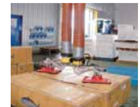
Use of vacuum lifts allows for safe and speedy transfer of even heavy cargo
